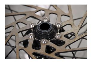
2. Ensure the hub mounting surface and threads are clean and debris-free. If dirty, clean using Isopropyl Alcohol (IPA) or dish soap and warm water. It is best to apply IPA or soapy water to a clean cloth or lint-free shop towel then wipe down the mounting face. Do not spray IPA directly onto the hub mounting face as IPA may work its way into the bearings etc.
